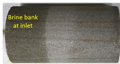
Fig. 1. Berea sandstone sample taken from test rig at the early stage of an imbibition Rel Perm measurement using standard, co-current SCAL methods. A large brine bank has formed at the inlet that blocks the permeability to gas.
