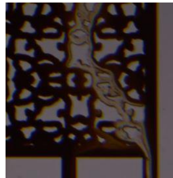
Fig. 9. Moment of breakthrough for the solvent finger in experiment 7 which has travelled through the matrix (see also figure 17).
