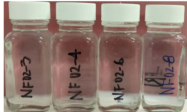
Fig. 6 Visual analysis of NPs stability. The white colour at the bottom of each ampule indicates the aggregated NPs. Stretched polymers in SSW were observed in NF02-4.
