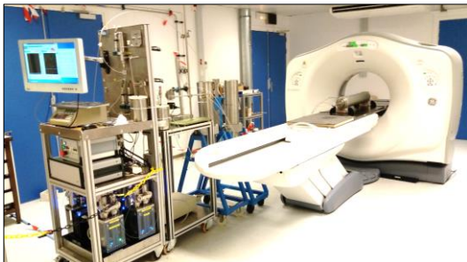
Fig. 1. Overview of the IFPEN medical CT Scan GEHC Discovery 750HD and the experimental setup
