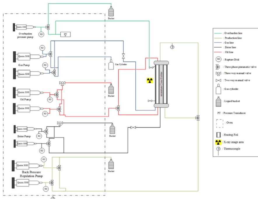
**Fig. 1** A schematic diagram of the experimental apparatus [19].
