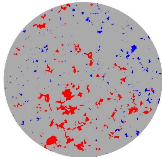
**Fig. 2** Pore-fluid occupancy map at the end of the drainage process (grain: gray, oil: red, and brine: blue).
