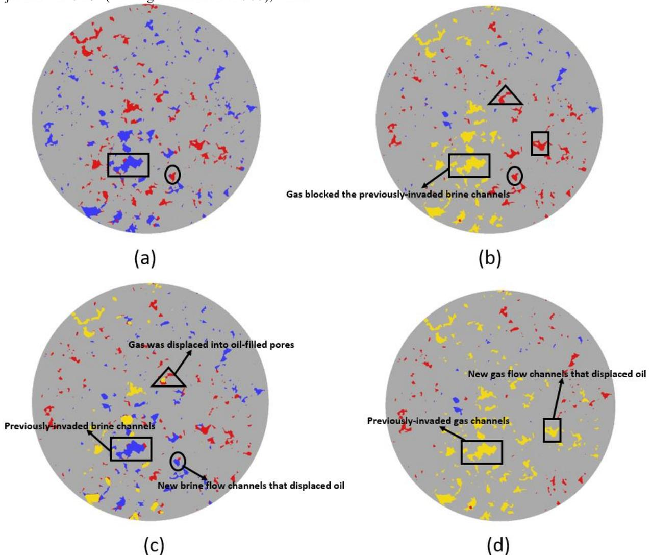
**Fig. 5** Two-dimensional cross-sectional views of in-situ fluid occupancy maps at the end of (a) the first cycle of waterflooding, (b) the first cycle of gas injection, (c) the second cycle of waterflooding, and (d) the second cycle of gas injection (grain: gray, gas: yellow, oil: red, and brine: blue).
