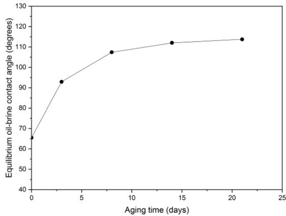
**Fig. 3** Variation of equilibrium oil-brine contact angle versus aging time (Thirty contact angles were measured at each date point).
