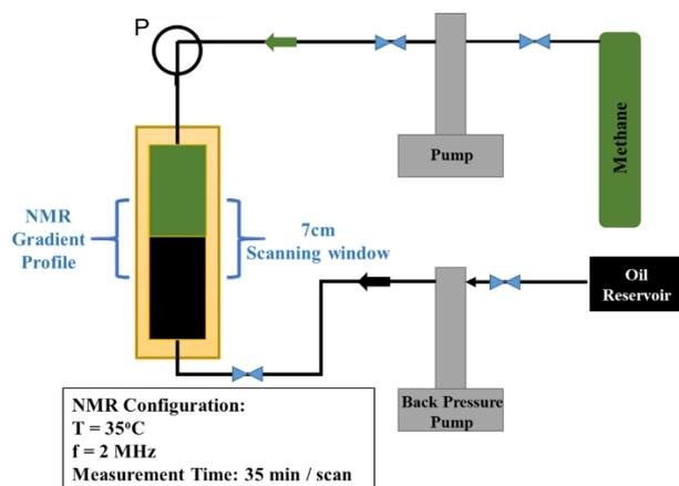
**Fig. 1.** Experimental setup, including NMR transparent  $ZrO_2$  pressure cell, placed within 2 MHz NMR spectrometer. The oil phase was injected from a downstream port; the gas phase was injected through an upstream port, with the pressure controlled
