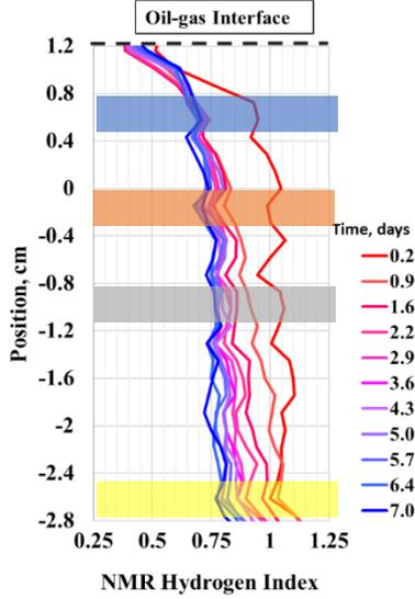
**Fig. 3.** HI profile within the oil phase as a function of time. The decreasing of the HI value within the oil phase is due to the methane diffusion. HI temporal profiles at different positions (color labels) within the oil phase are plotted in **Fig. 4**.
