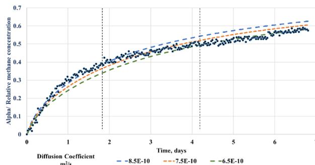
**Fig. 6.** The fitting of diffusion coefficient using the relative methane concentration profile. The diffusion rate can be precisely fitted within 25% of error, despite the experimental artifact, which makes diffusion rate decreases when gas molecules approach the end of the test cell.
