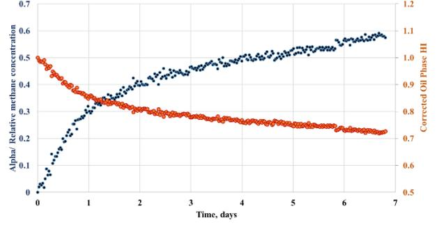
**Fig. 5.** The integral of HI respective to position, plotted as a function of time (red). Calculated relative methane concentration is also plotted (blue). The data is used to estimate methane diffusion coefficient.
