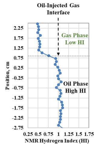
**Fig. 2.** An HI profile across the oil-gas interface. The position values are based on the relative position of the test cell in the NMR scanning window. The contrast in HI between the gas (low value) and the oil (high value) phases, allows to determine the dynamic position of the oil-gas interface during the experiment.
