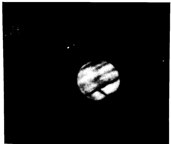
Figure 20. An end view scan of a core plug taken from a section of laminated sand reveals fractures in the plug.
