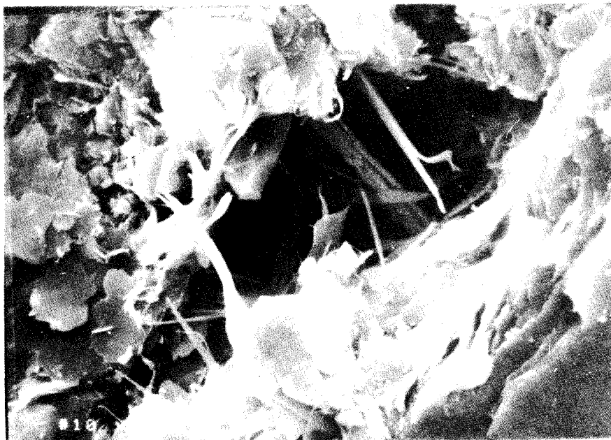
Figure 6. Photomicrograph of convection oven dried core sample from 3,530 feet, showing well developed fibrous illites (2,400 X). Long dimension of photo is 50 microns.
