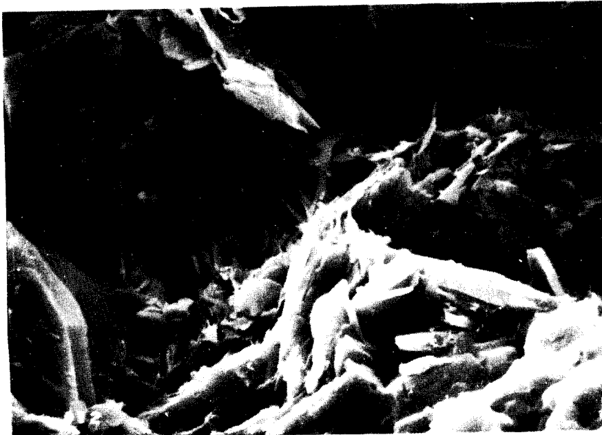
Figure 5. Photomicrograph of freeze dried core sample from 3,530 feet, showing well developed fibrous illites (2,400 X). Long dimension of photo is 50 microns.
