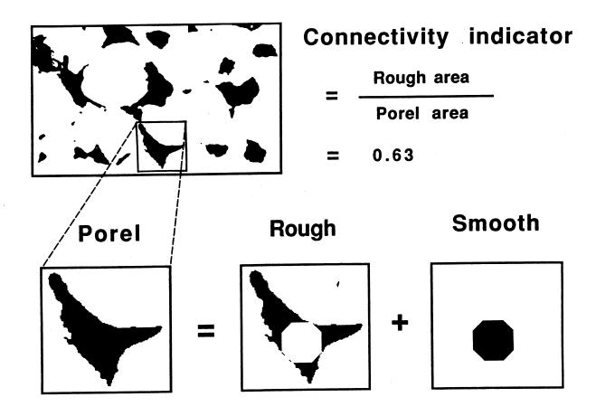
Figure 4.- A porel (pore element) is a discrete unconnected patch of porosity. The smooth component is the portion with the largest size which resembles an inscribed circle of the porel. The rest of the porel is rough component. The ratio of the rough component to the porel area is defined as a connectivity indicator.
