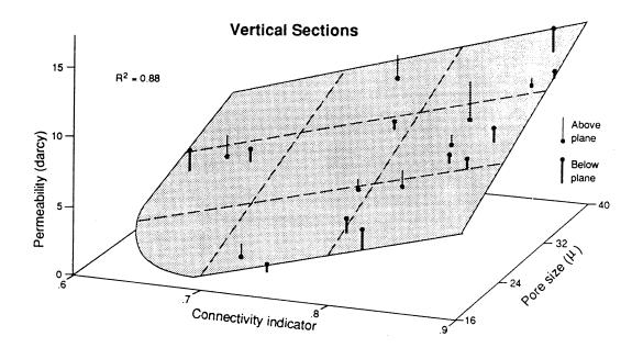
Figure 7.- Regression surfaces with pore size and connectivity as independent variables, and permeability as dependent variable. Solid circles are the data projected on the surfaces (predictions) and vertical lines indicate the distances between data points and their projections (residuals).
