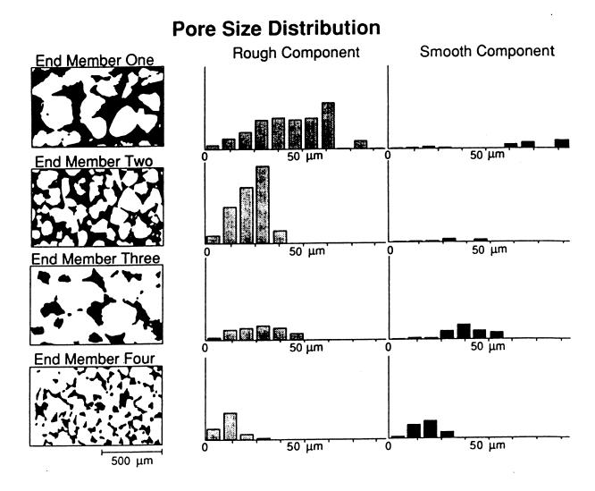
Figure 6.- Representative end member images with their rough and smooth size distributions. The mean pore sizes of the four images are 45, 22, 31, and 13.5 microns; and the connectivity indicators are 0.90, 0.96, 0.59, and 0.53 respectively.
