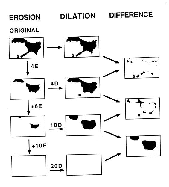
Figure 2.- Erosion-dilation image processing algorithm. Dilated images represent a sequential loss of porosity from small features to large features. This is used as a size distribution by measuring the differences between subsequent dilated images.
