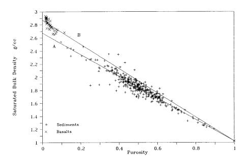
FIGURE 3 Porosity - bulk density plots.
