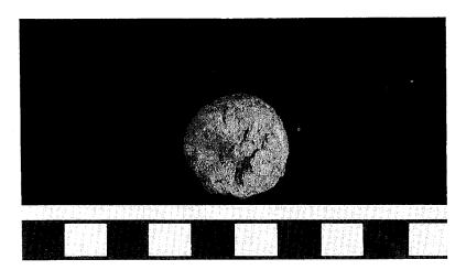
FIGURE 1. Percussion sidewall core. Scale in centimeters.
