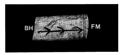
FIGURE 2. Rotary-drilled sidewall core. The borehole end (BH), formation end (FM), groove cut by the diamond drill bit (G) and line marking the top of the core are shown.
