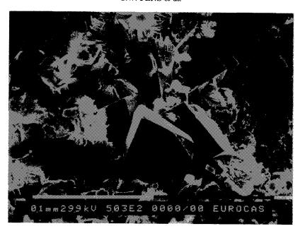
FIGURE 1 SEM secondary electron image showing surface structure of a shaly sandstone at 500 X magnification. The white scale bar is 100  $\mu m.$  Note the kaolinite booklets upper left and the dolomite rhombs in the centre.
