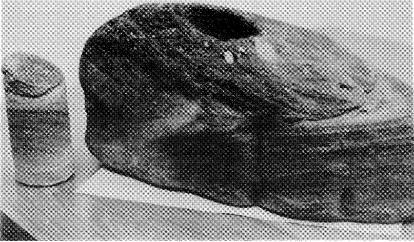
FIGURE 7 Fluvial crossbedded coarse sandstone sample from Burghead from which a 3,25 inch (8cm) core sample was cut. Sample is 23cm. high.
