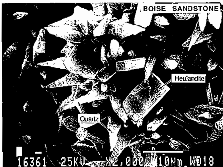
FIGURE 10 Scanning electron photomicrograph of Boise sandstone core.
