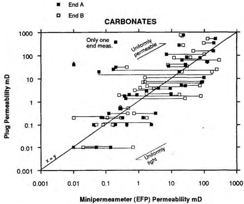
Fig 7. Comparison between the minipermeameter data measured on each end of a plug and the equivalent plug analysis permeability.
