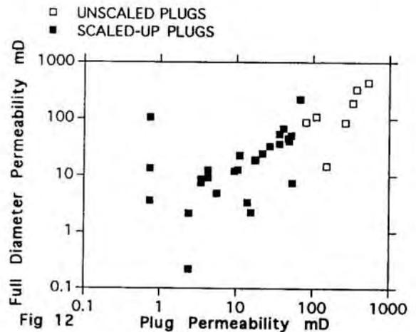
Figs 11 and 12. Correlation between full diameter and plug permeabilities for carbonate samples below 80 mD (Fig 11) can be used to scale up low permeability plug data (Fig 12).
