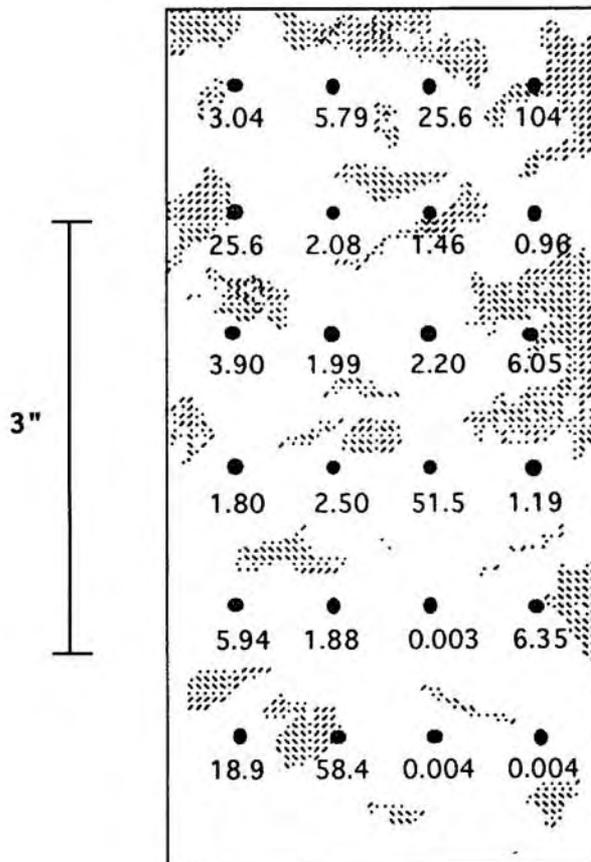
Fig 10. Minipermeameter measurements illustrate the permeability heterogeneity of mottled siltstones.
