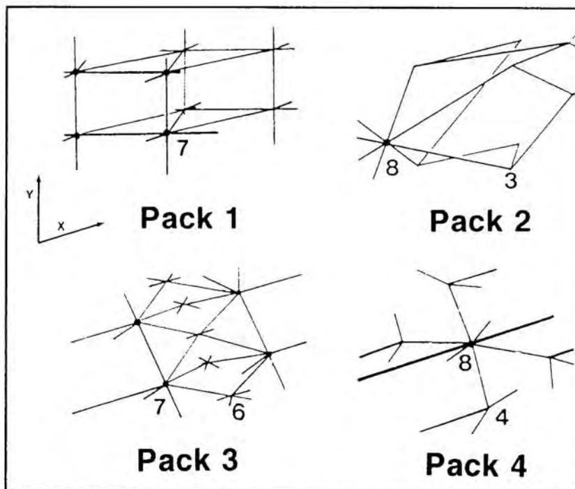
**Figure 4-** Equivalent networks of the void space of packs of spheres. The numbers are the coordination number of the pores.
