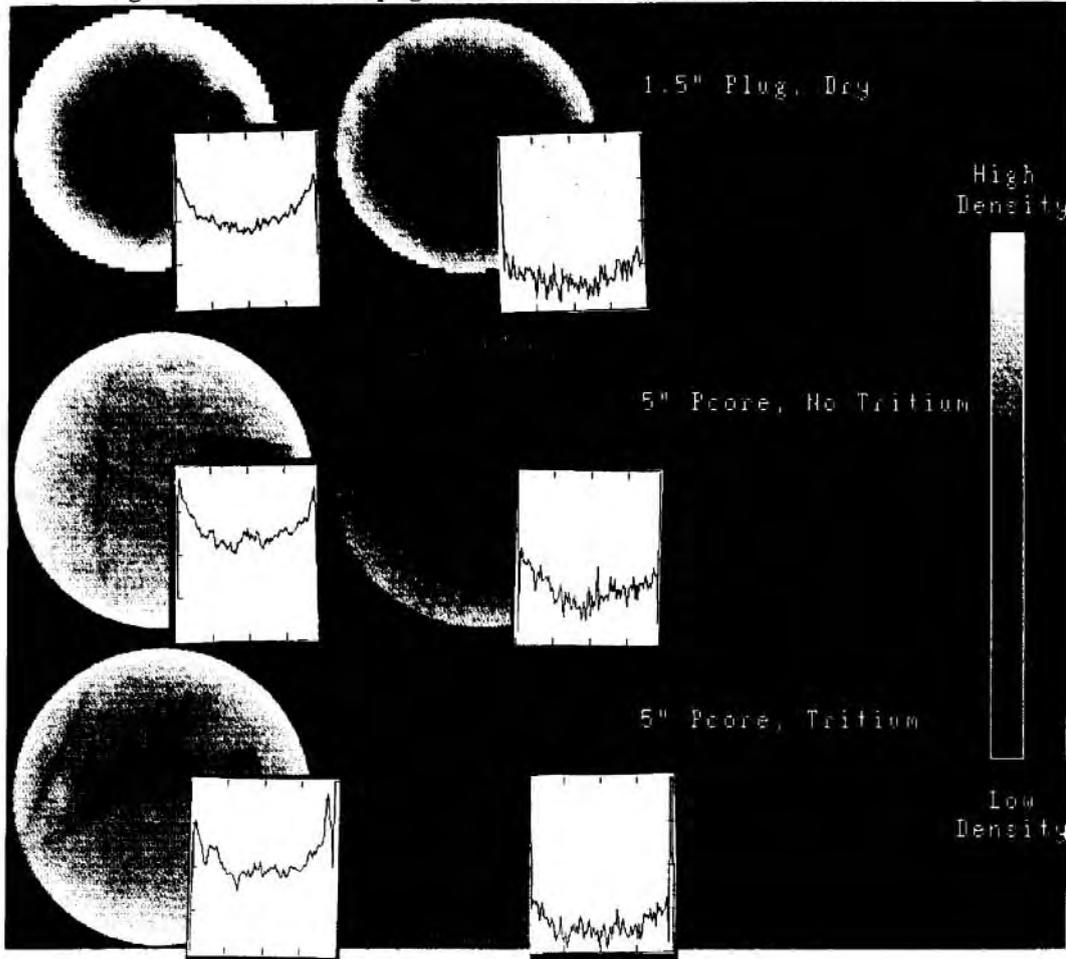
Fig. 2 - CT scans of core samples scanned in air (left) and under water (right).
