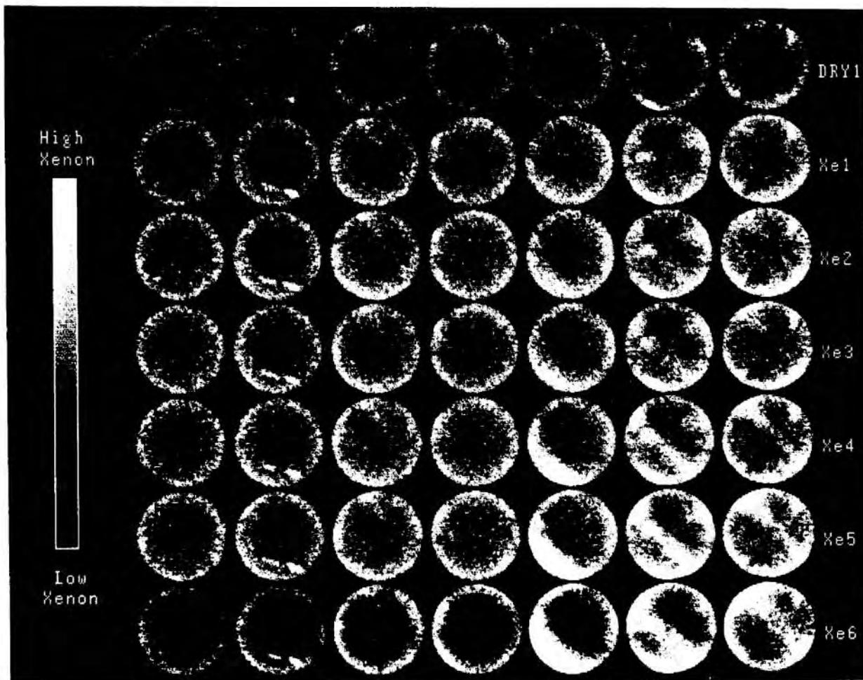
Fig. 5 - CT investigation of drilling fluid transport by vapor convection.
