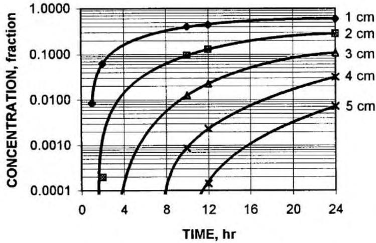
**Fig. 4 - Calculated Invasion Depth by Vapor Convection**
