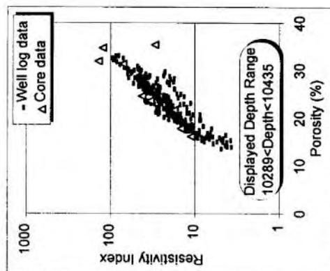
Figure 10: Comparison of laboratory and well log resistivity indices at initial water saturations with porosity.
