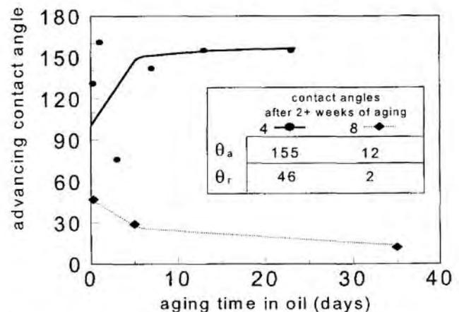
Figure 2. Adsorption of A-93 crude oil with 0.1 M NaCl brines on glass at 80°C.
