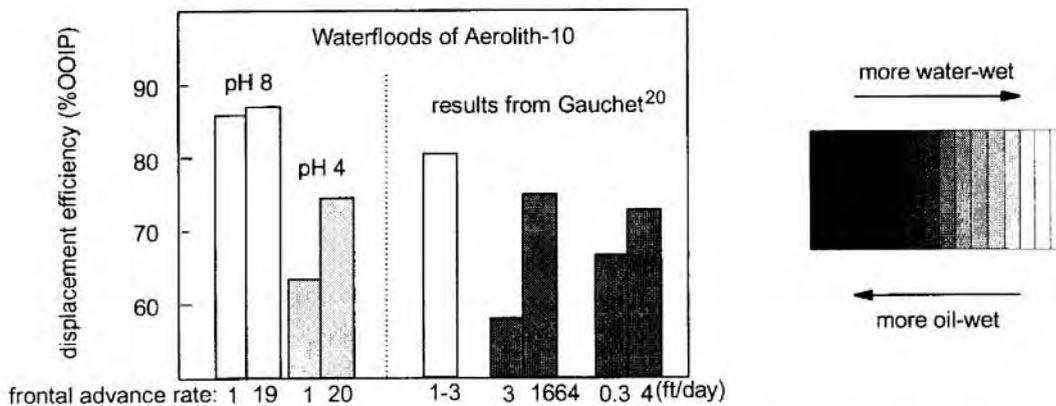
Figure 7. Waterflood displacement efficiency for different wetting conditions and frontal advance rates in Aerolith-10.
