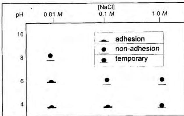
Figure 1. Adhesion of A-93 crude oil with NaCl brines on glass at 80°C.
