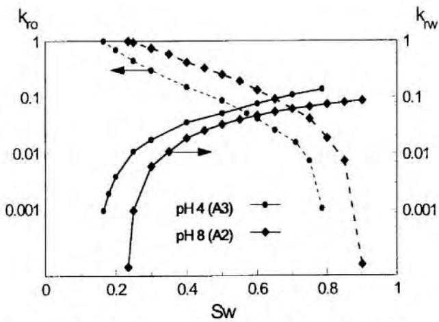
Figure 5. Relative permeabilities from fits to high rate waterfloods of Aerolith-10.
