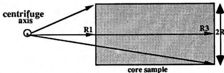
**Figure 1 :** Top view of the centrifuge geometry.
