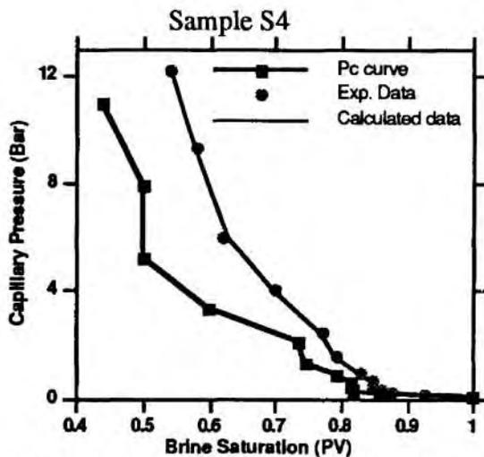
**Figure 7:** Calculated Pc curve for the St Maximin limestone in experiment 2 (the less porous face at the largest radius of rotation).
