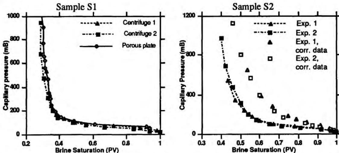
Figure 3: Calculated  $P_c$  curves with correction for radial effect. Exp. 1 and 2: centrifuge experiments at a small and large radius respectively (table 1). Left (sample S1): the two centrifuge experiments agree with the Porous Plate measurements. Right: the same  $P_c$  curves are found and the corrected experimental data are identical.
