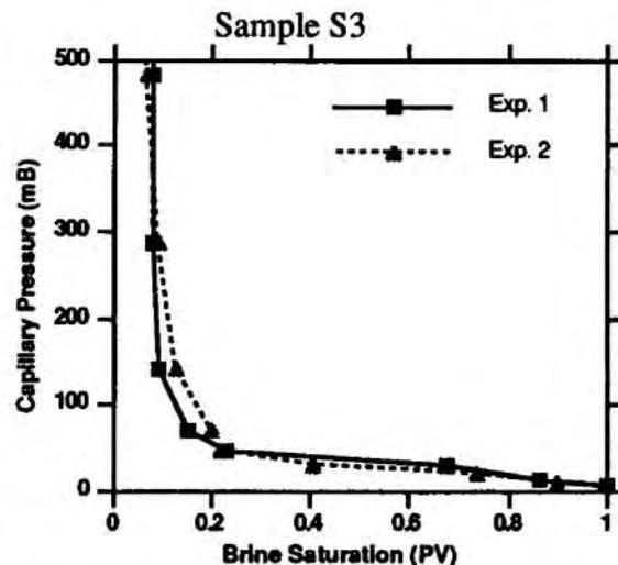
**Figure 6:** comparison between Pc curves from the experiment 1 and 2. Case of a lamination nearly parallel to acceleration.
