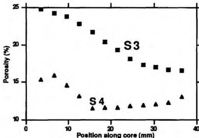
**Figure 4:** porosity profile for the Fontainebleau sandstone (S3) and the St Maximin limestone (S4) samples. S3 and S4 have a lamination nearly parallel and perpendicular to the centrifuge acceleration, respectively.
