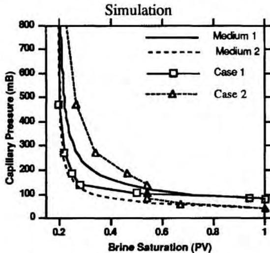
**Figure 9:** Interpretation of simulated centrifuge data with a heterogeneous sample. In case 1, the medium 1 is the closest to the axis of rotation.
