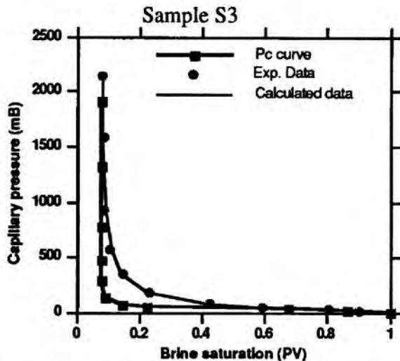
**Figure 5:** Calculated Pc curve for the Fontainebleau sandstone in experiment 1 (the most porous face at the largest radius of rotation).
