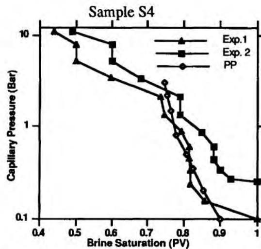
**Figure 8:** Pc curves (air-brine) from centrifuge experiment 1, 2 and porous plate (PP). Case of a lamination perpendicular to acceleration.
