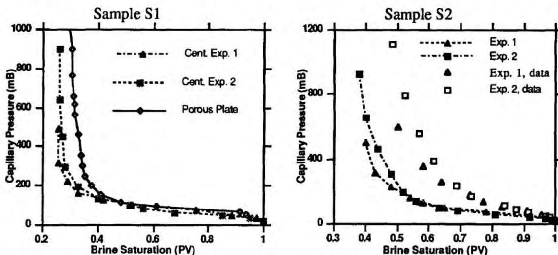
**Figure 2:** Calculated Pc curves without correction for radial effect. Exp. 1 and 2: centrifuge experiments at a small and large radius respectively (table 1). Left (sample S1): the two centrifuge experiments yield different Pc curves, both different from the Porous Plate curve. Right: different Pc curves are found as a result of different data  $\{\bar{S}, P_{C1}\}$ .
