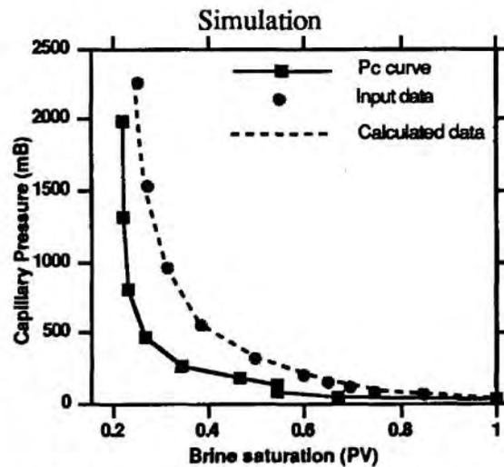
**Figure 10:** Calculated Pc curve from simulated centrifuge data, case 2 (medium 2 closest to the axis of rotation).
