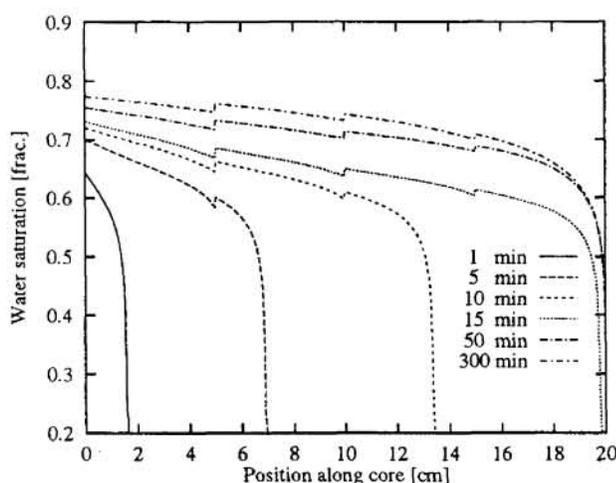
Figure 17: USS saturation profiles with capillary pressure. Ordering 1234.
