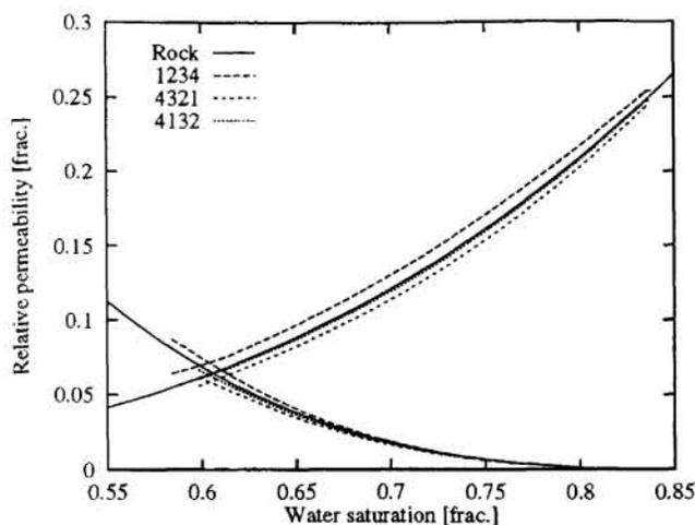
Figure 16: USS relative permeabilities without capillary pressure.
