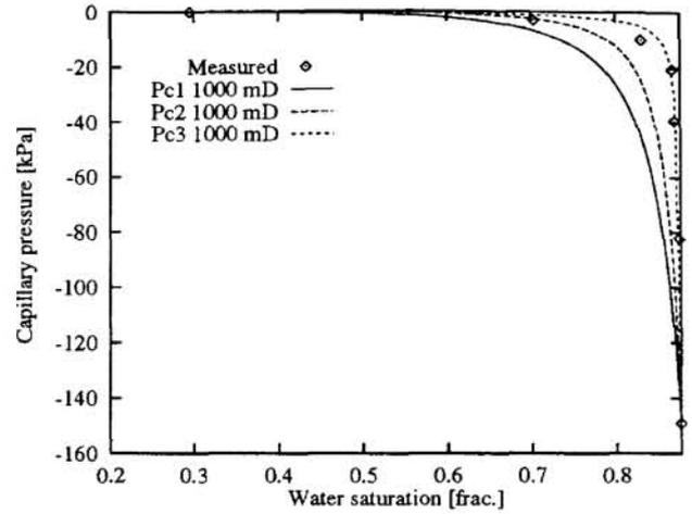
Figure 12: 1000 mD capillary pressure curves for three different Leverett-J functions.
