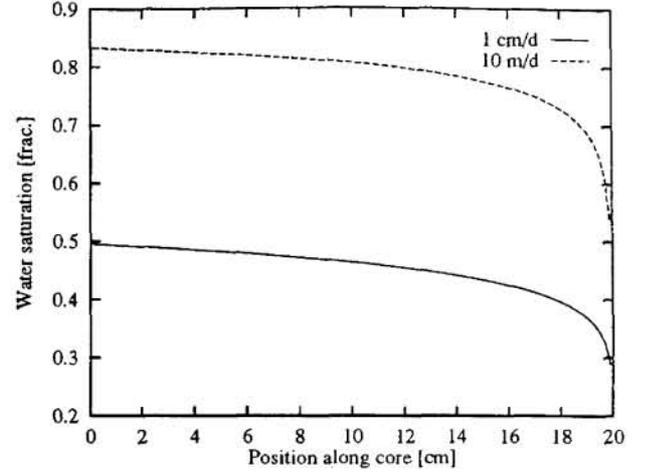
Figure 1: Saturation profiles ( $f_w = 1$ ) in a homogeneous 1000 mD core at different rates.
