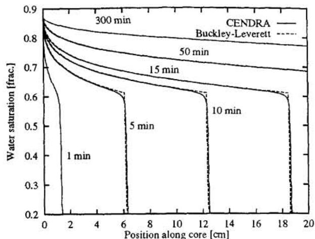
Figure 15: USS saturation profiles without capillary pressure. Other properties as the base.
