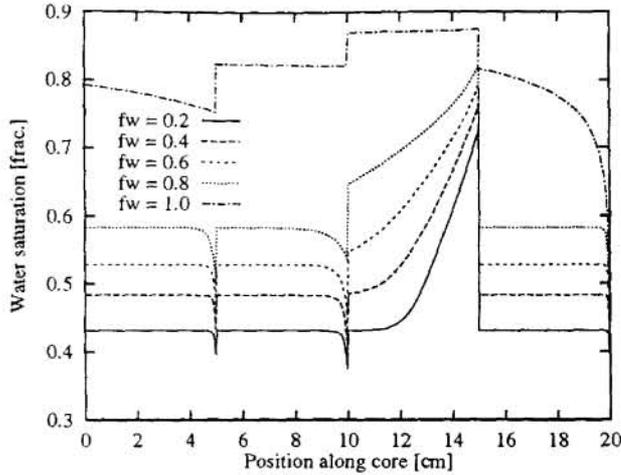
Figure 8: Steady state saturation profiles for the extreme permeability variation case. Ordering 2341.
