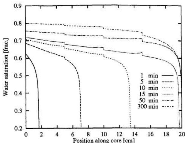
Figure 18: USS saturation profiles with capillary pressure. Ordering 4321.
