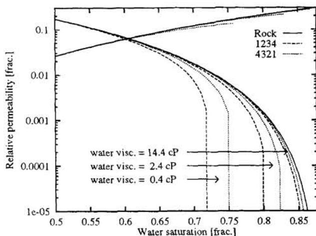
Figure 14: SS relative permeabilities for different water viscosities. Oil viscosity is always 2.4 cP.
