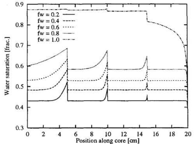
Figure 7: Steady state saturation profiles for the extreme permeability variation case. Ordering 4321.
