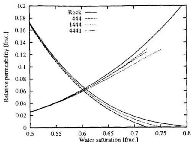
Figure 13: SS relative permeabilities for different composite cores made of three 6 cm, 1000 mD cores and one 2 cm, 400 mD core.
