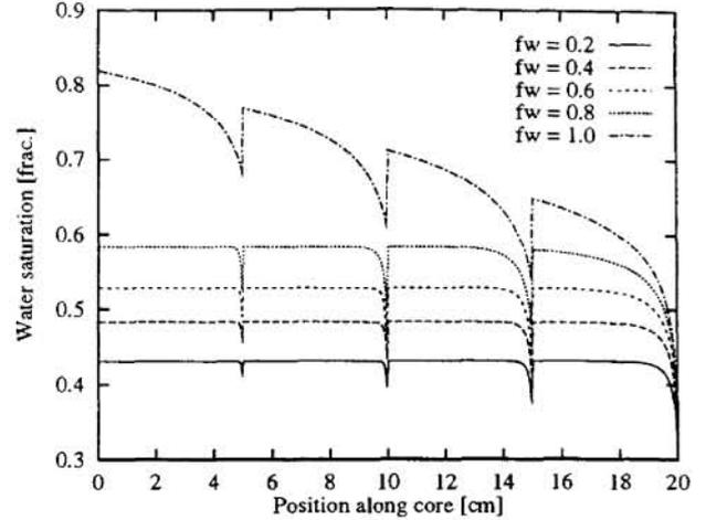
Figure 6: Steady state saturation profiles for the extreme permeability variation case. Ordering 1234.
