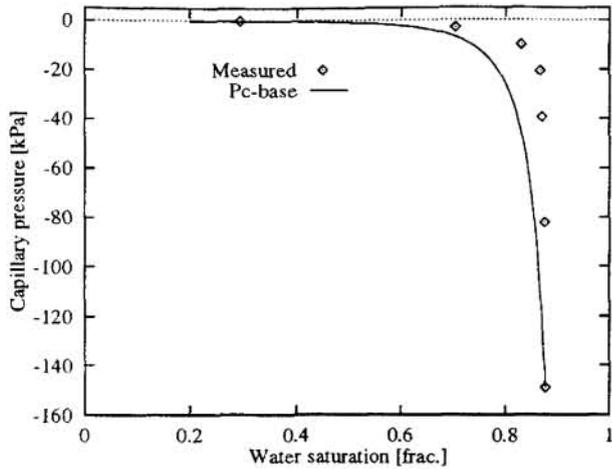
Figure 5: The capillary pressure used as a basis in this analysis. Also shown are measured data from a typical North Sea reservoir.
