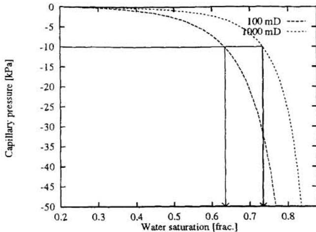
Figure 3: Capillary continuity causes a saturation jump between two neighbour cores.
