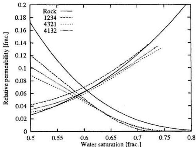
Figure 19: USS relative permeabilities with capillary pressure.
