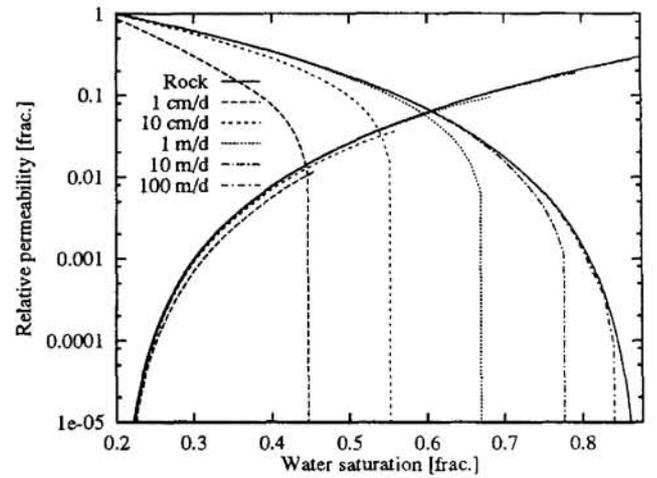
Figure 2: Steady state relative permeabilities for different Darcy velocities. Homogeneous 1000 mD rock.
