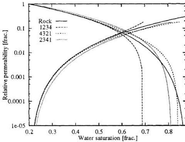
Figure 9: Steady state relative permeabilities for different compositions of the extreme permeability variation case.
