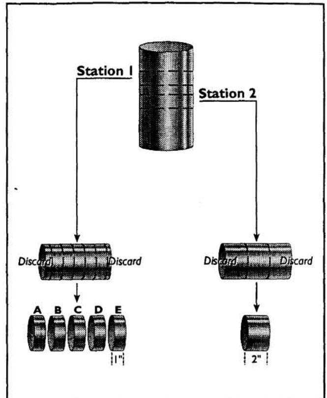
Figure 6 Plugs cut from Low Invasion Core
