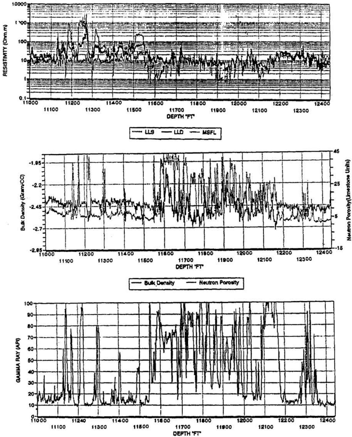
Fig. 2 Log data record for shaly sand sections, well 1, ( SUCO documents )
