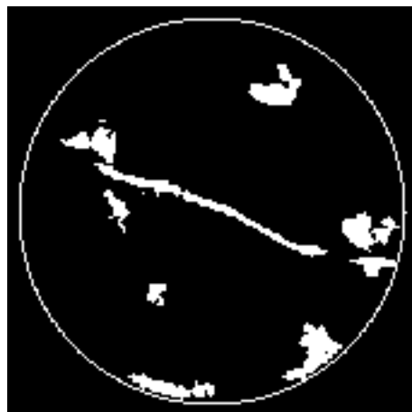
Figure 5b. Slice 5: the mask for computing the constituent porosity
