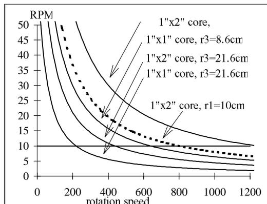
Figure 8 : Equivalent error in rotation speed, when neglecting gravity correction in imbibition centrifuge measurements.
