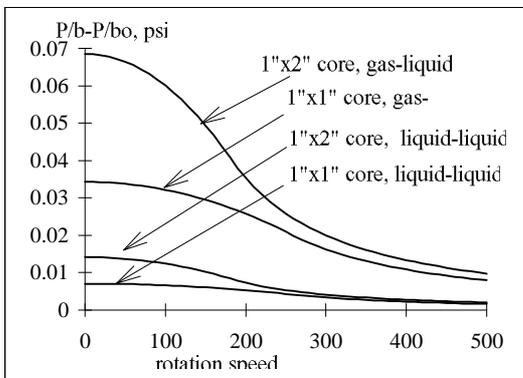
Figure 5 : Extension of gravity correction to pressure, drainage measurements. The maximum value is in the range of the gravity capillary pressure along the height of the core :  $2 \Delta \rho gR$
