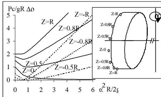
Figure 2 : Evolution of Pc on the border of the outlet face during a centrifuge drainage. By effect of gravity, Pc may be decreasing when the rotation speed is increased. The gray area displays the core zone where such reverse variation of Pc may occur. That zone is usually much less than 1% of the core volume.
