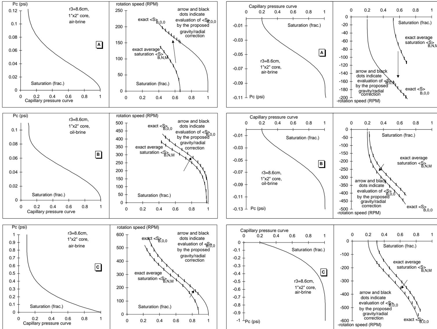
Figure 3 : Evaluation of the proposed gravity/radial correction in drainage.
