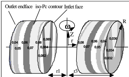
Figure 1 : The Centrifuge geometry. Core samples are rotated around a vertical axis. The actual capillary pressure distribution is drawn for a 2"x2" core with an air-brine system rotating at 100 RPM at  $r_3=8.6\text{cm}$ . Iso-Pc are indicated in psi.
