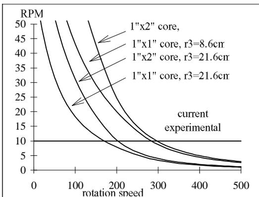
Figure 7 : Equivalent error in rotation speed, when neglecting gravity correction in drainage centrifuge measurements.
