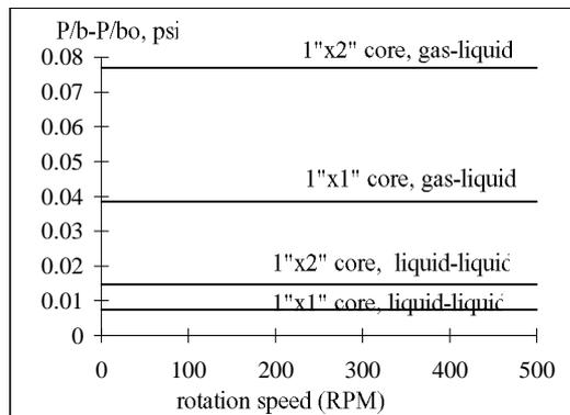
Figure 6 : Extension of gravity correction to pressure, for imbibition measurements. The maximum value is in the range of the gravity capillary pressure along the height of the core :  $2 \Delta \rho gR$
