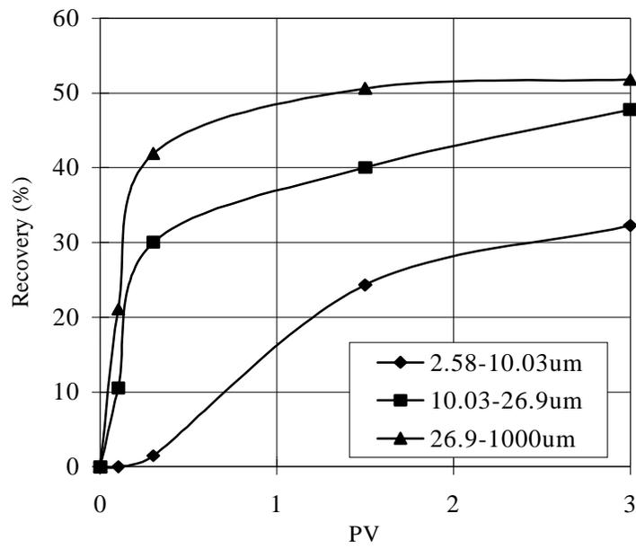
Fig.8 Oil recovery of different sized pores in core plug No.1 at different water injection stages
