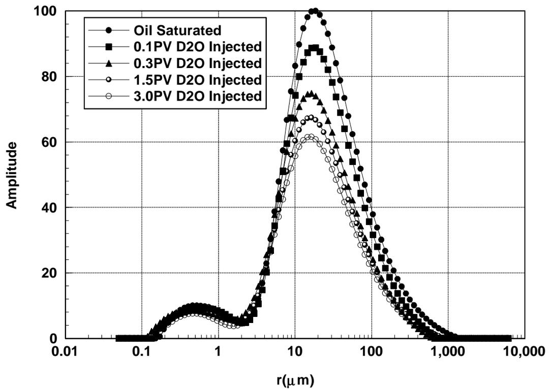
Fig.6 Oil distribution of core plug No.3 at different water injection stages
