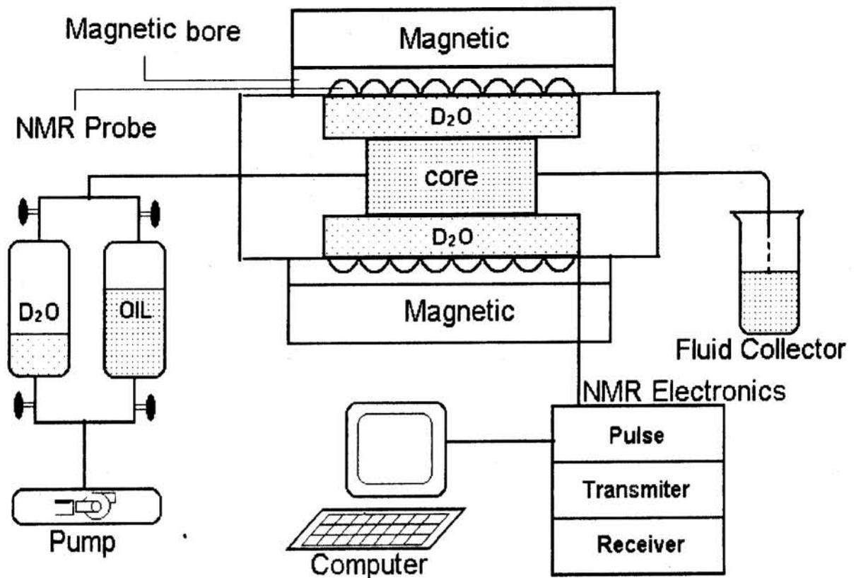
Fig.1 The sketch map of NMR Waterflooding System
