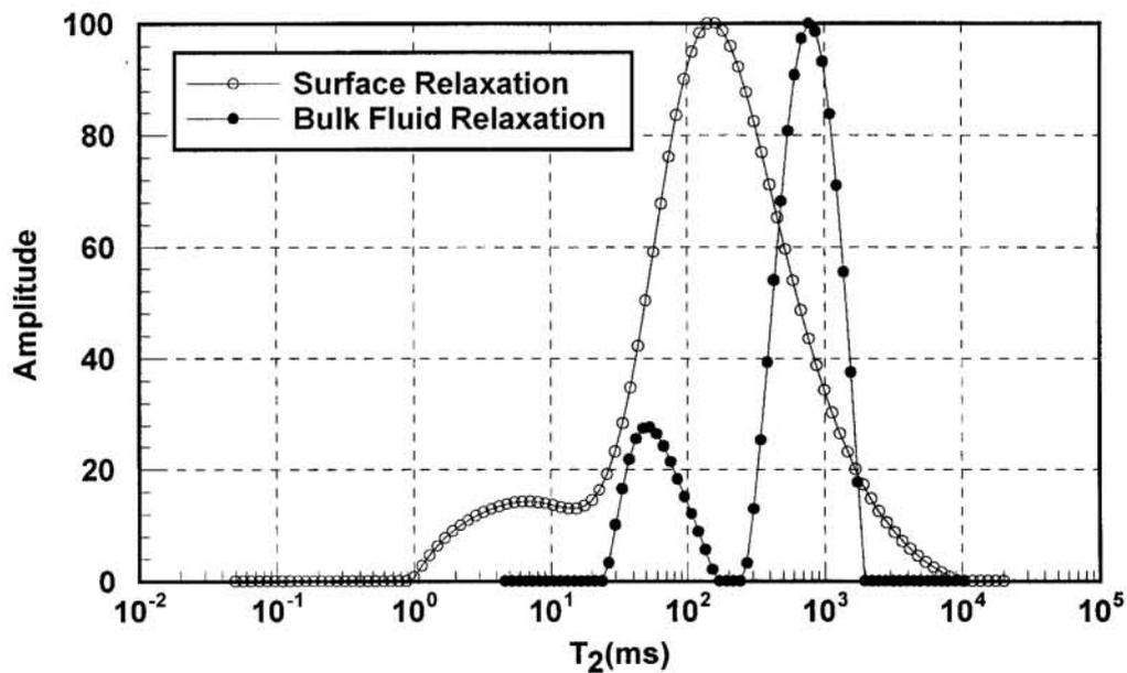
Fig.2 Comparison of bulk fluid relaxation and surface relaxation for core plug No.4
