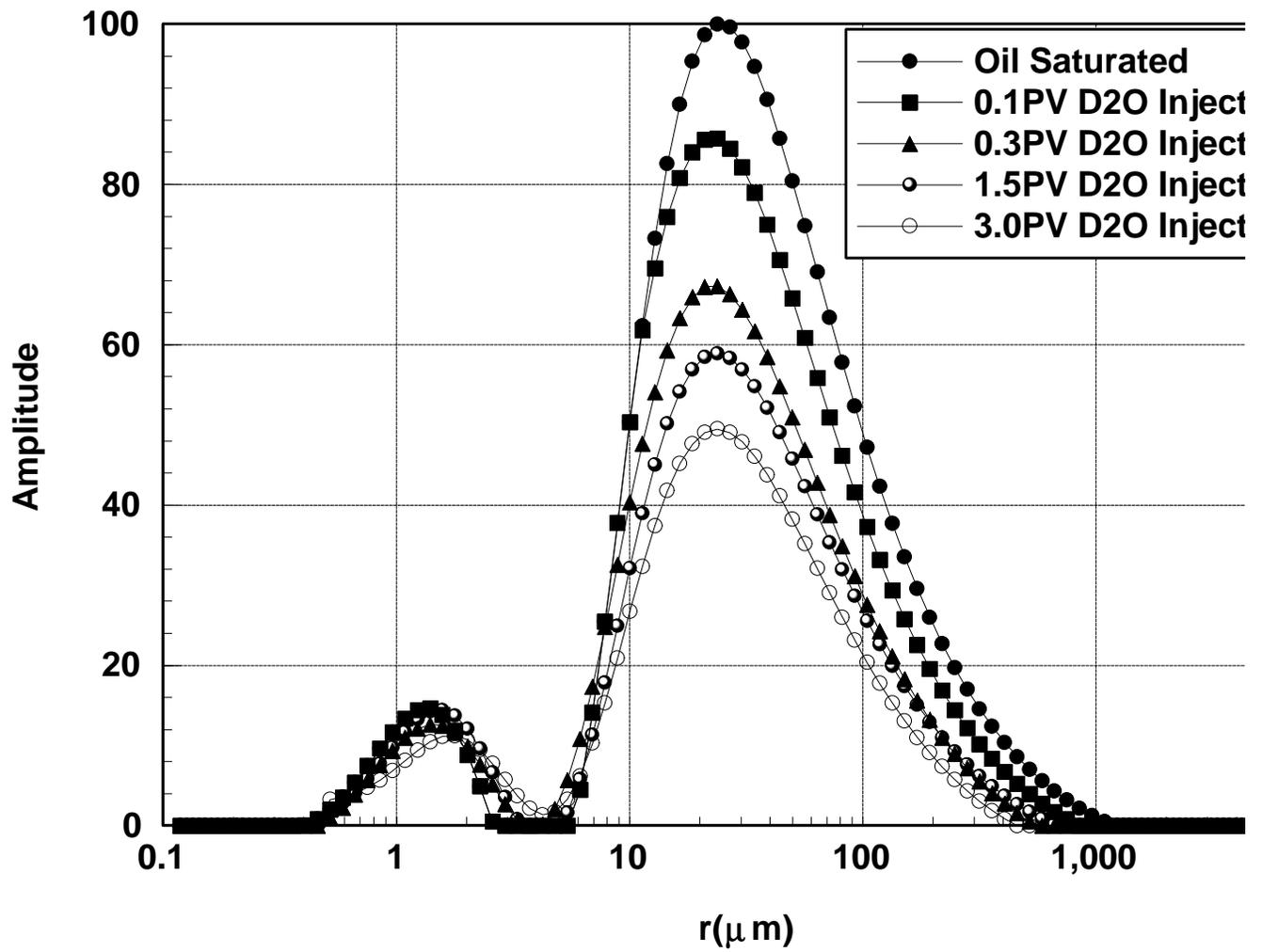
Fig.4 Oil distribution of core plug No.1 at different water injection stages
