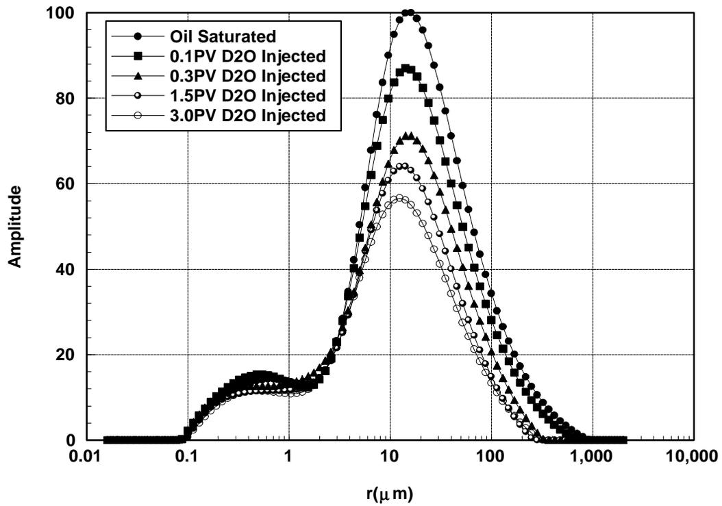
Fig.7 Oil distribution of core plug No.4 at different water injection stages
