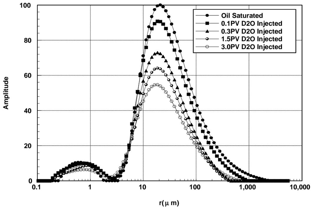
Fig.5 Oil distribution of core plug No.2 at different water injection stages
