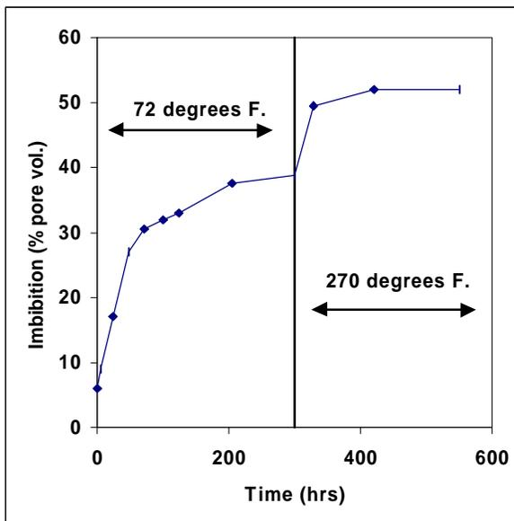
Figure 3: A spontaneous water imbibition test that was conducted with stock tank crude oil in chalk at ambient and reservoir temperature illustrates sensitivity to test temperature.
