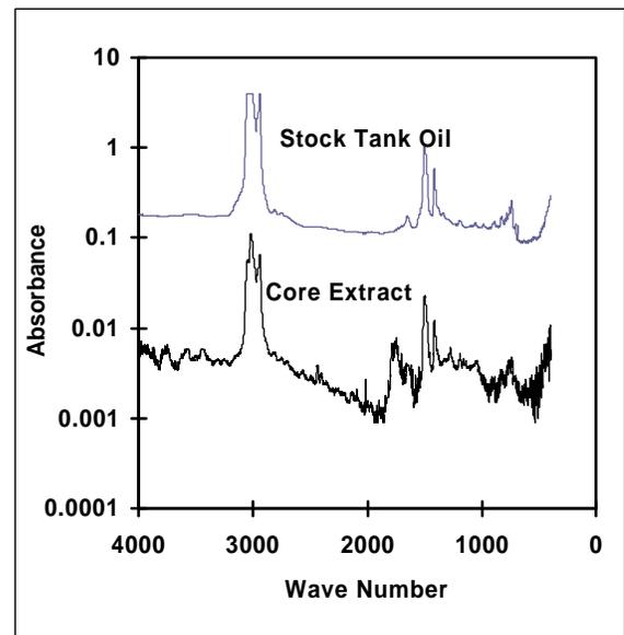
Figure 4: A comparison of infrared absorbance spectra shows that the toluene removes crude oil from reservoir chalk core plugs.
