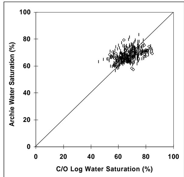
Figure 8: The comparison between different interpretation methods showed general agreement for the near well bore saturations of a waterflood zone.
