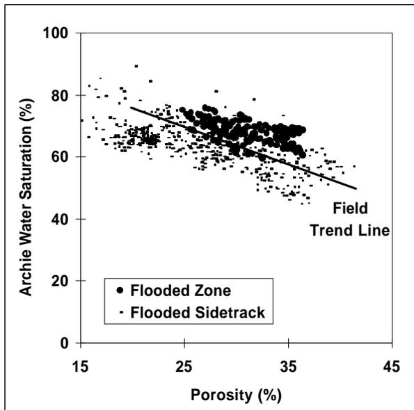
Figure 11: Interpretation away from the near well bore showed a decreasing water saturation with porosity in waterflooded zones. The line indicates the direction of the trend.
