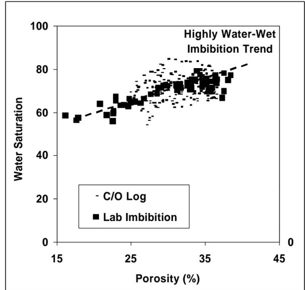
Figure 10: The near well bore in the water flooded zone exhibited the same trend as observed in the laboratory for highly water-wet chalk which are the upper most data points of set 2.
