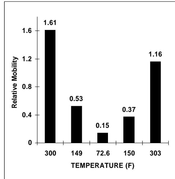
Figure 2: Fluid mobility as measured in porous rock is shown with measurements proceeding time-wise from left to right. A permanent loss in mobility can be seen after cooling to ambient temperature.
