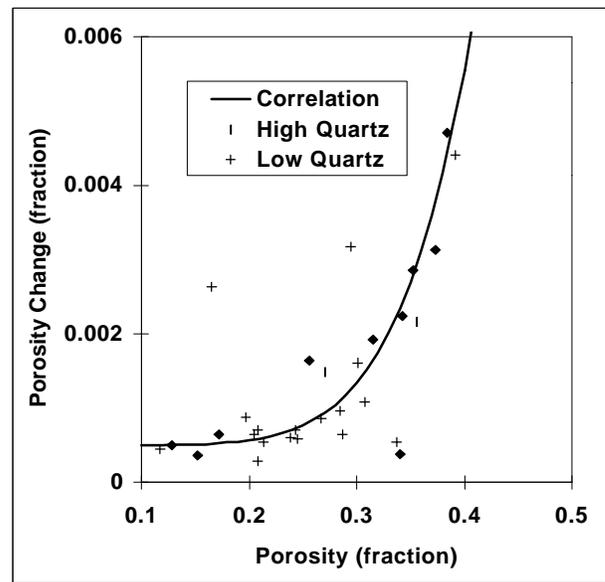
Figure 6: The porosity of the chalk varies with the change in stress from ambient to reservoir pressures with the higher porosity chalk showing greater decreases.
