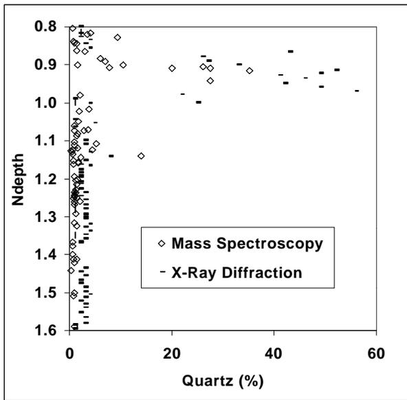
Figure 5: The quantity of quartz in the chalk varies with normalized well depth (Ndepth) in the reservoir.
