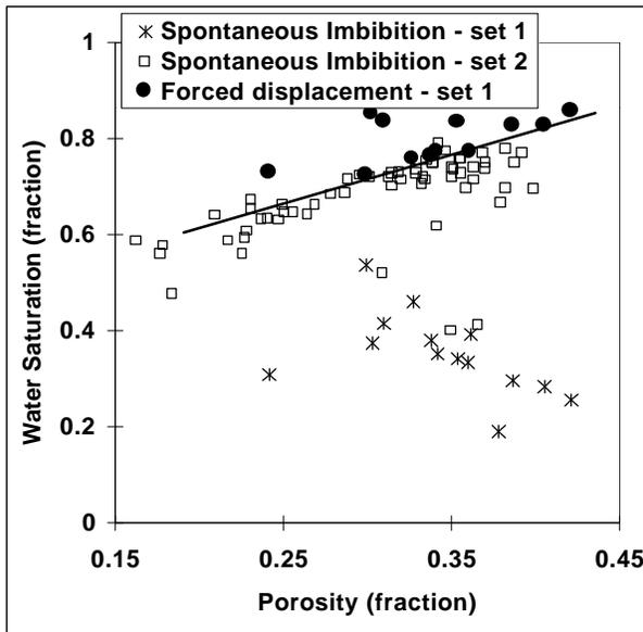
Figure 7: Laboratory tests established the saturation behavior of reservoir chalk plugs with displacement mechanism. The line is the trend for highly water-wet spontaneous imbibition and forced imbibition.
