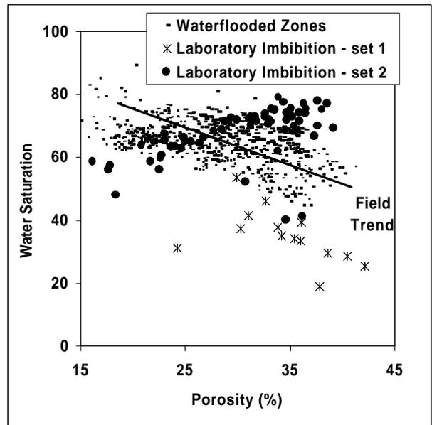
Figure 12: Comparison of laboratory imbibition measurements with field reservoir behavior show different trends and water saturations.
