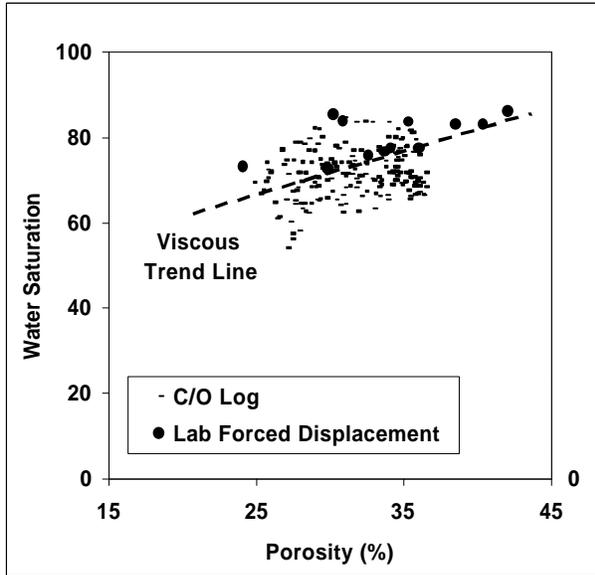
Figure 9: The near well bore in the water flooded zone exhibited the same trend as observed in the laboratory for forced imbibition (forced/viscous displacement) from data set 1.
