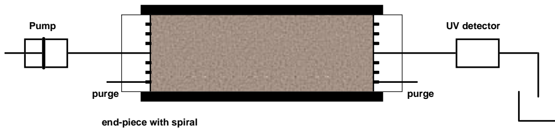
Figure 5: Schematic of the experimental set-up. Injection end-pieces are equipped with spirals to flush both inlet and outlet line. The outlet line is as short as possible. A confining pressure of 55 Bar was applied.
