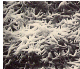
Fig. 2 Photomicrograph of North Burbank sand grain showing chlorite coating (adapted from Trantham and Clampitt, 1977).
