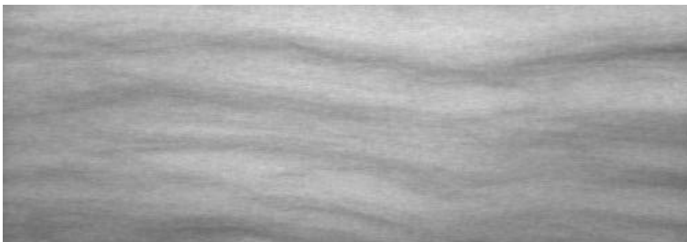
FIGURE 4. X ray image of a slab of Bluejacket sandstone showing significant heterogeneity.
