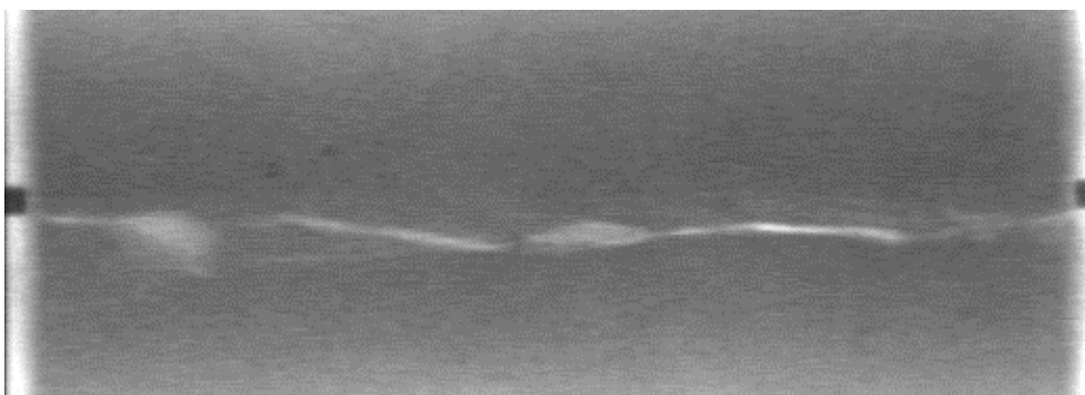
Figure 7 X-ray image of the fractured Kansas outcrop chalk plug showing position of the inlet and outlet ports (the dark spots at the ends of the plug).
