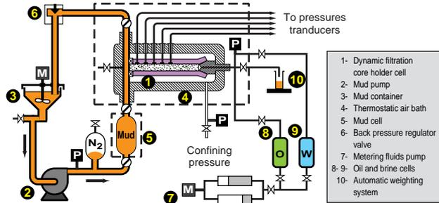
Figure 3: Equipment for dynamic mud leak-off tests on long core samples.
