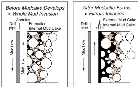
Figure 2: Drilling fluid invasion and filter cake formation.
