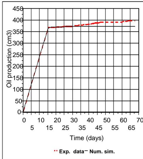
Figure 2. Oil production from the column.
