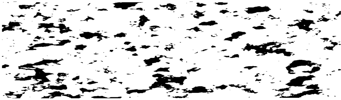
Fig.7 – Point count porosity=9%, Log porosity=18%
