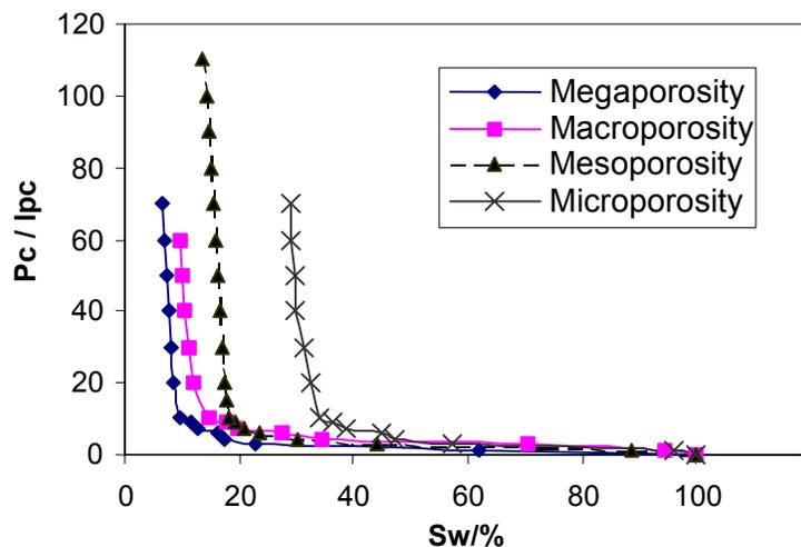
**Figure 1.** Capillary pressure curves for core plug samples of different rock types.
