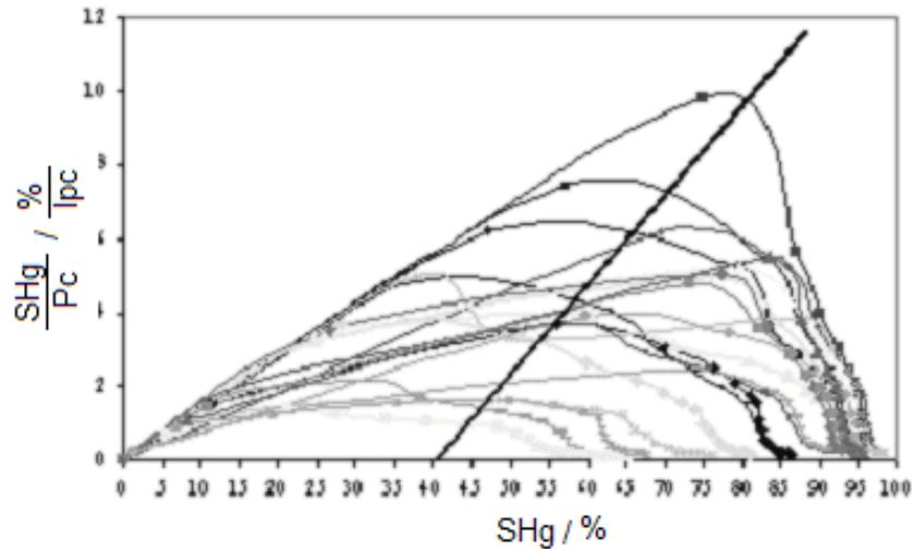
**Figure 2.** Apex method for determining pore throat radius.
