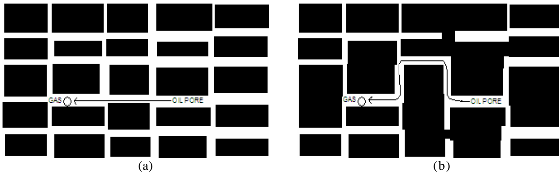
Figure 5. In the well connected system (a) diffusion acts more effectively in transporting dissolved gas from the oil pore into the gas bubble. In (b) the path of diffusion is more tortuous and the pore will become highly supersaturated at the point in the depletion
