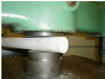
Figure 1: Fracturing the core in the laboratory.
