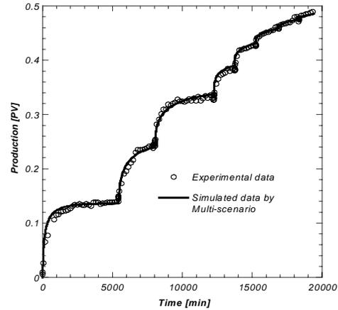
**Figure 14:** Reconciliation of the multi speed centrifuge experiment.
