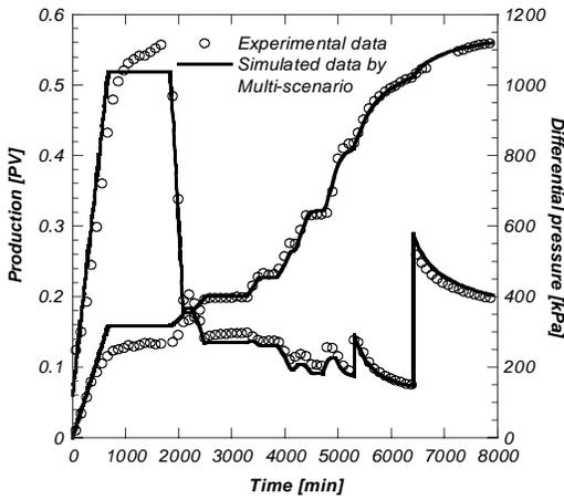
**Figure 13:** Reconciliation of the steady state experiment.
