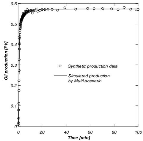
**Figure 3:** Reconciliation of the single speed centrifuge data.
