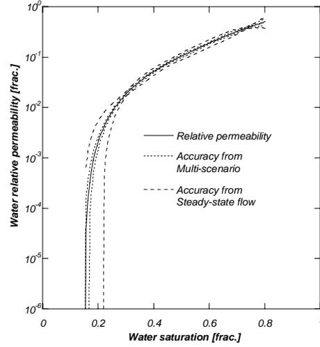
**Figure 5:** Water relative permeability from steady state data and multi-scenario estimation.
