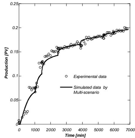
**Figure 18:** Reconciliation of the multi speed centrifuge experiment.
