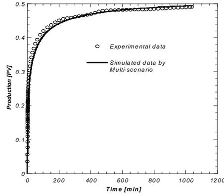
**Figure 12:** Reconciliation of the single-speed centrifuge experiment.
