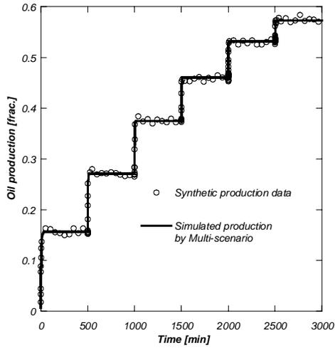
**Figure 4:** Reconciliation of the multi speed centrifuge data.
