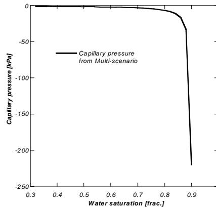
**Figure 11:** Estimated capillary pressure using the multi-scenario feature.
