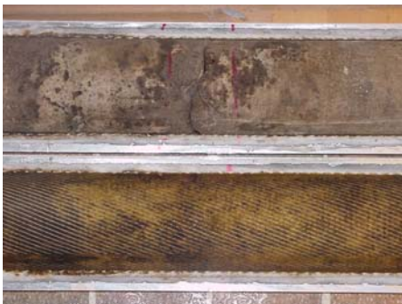
Figure 5- Sliced Core barrel (bottom) and core (top) illustrating sponge-core oil capture effectiveness
