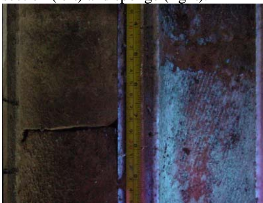
Figure 7- UV Photo of sponge section showing mud cake formation
