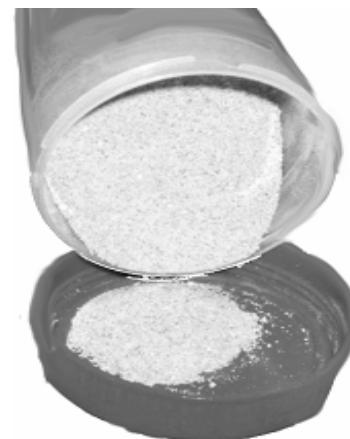
Figure 2. Loose sand material used to prepare the synthetic plugs.
