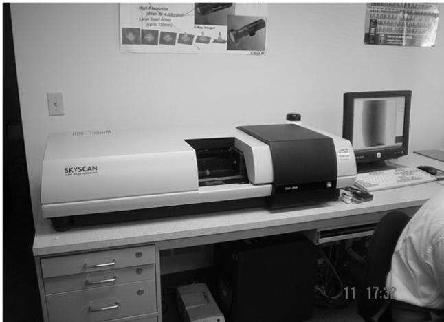
Figure 1 – Skyscan 1072  $\mu$ -CT system used to study the sandstone samples. The equipment is simple to operate and the resolution depends on sample size and composition.
