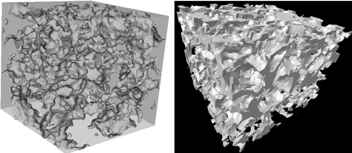
Figure 8 - Visualization of the porous medium as a result of the 3-D stochastic reconstructed model (left) and as depicted by the  $\mu$ -CT analysis (right).
