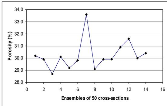
Figure 5 – Porosity profile of groups with 50 cross-sections of the Botucatu sample (190  $\mu\text{m}$  intervals) showing a porosity total average of 30.2%.
