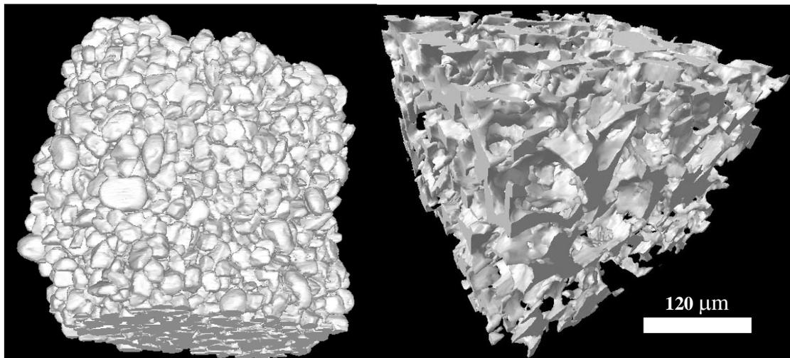
Figure 3 – Left: 3-D  $\mu$ -CT image showing part of the sample grains in light gray. Right: a cubic section of the same  $\mu$ -CT volume showing the pore space in light gray. The pixel resolution in both images is 3.8  $\mu$ m. Average grain size fraction is fine to medium sand.
