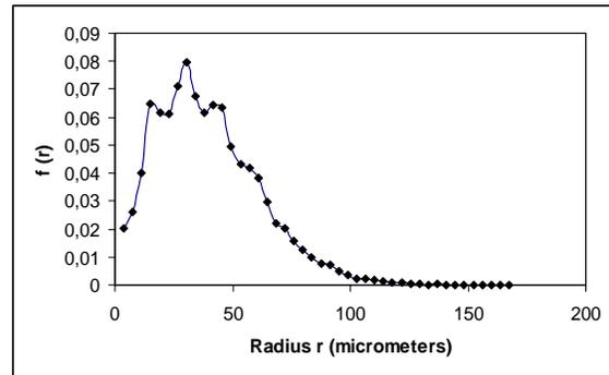
Figure 6 – Average pore size distribution of the 50 groups of  $\mu$ -CT cross-sections, showing a frequency peak in the 30  $\mu\text{m}$  size.
