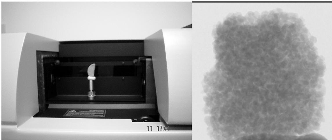
Figure 2 – Left: detail of the Skyscan 1072  $\mu$ -CT system showing sample chamber and holder with a half plug head. The best resolution was achieved using a smaller sample (bulk sample X-ray image to the right), about 1/5 in volume of the one shown to the left.
