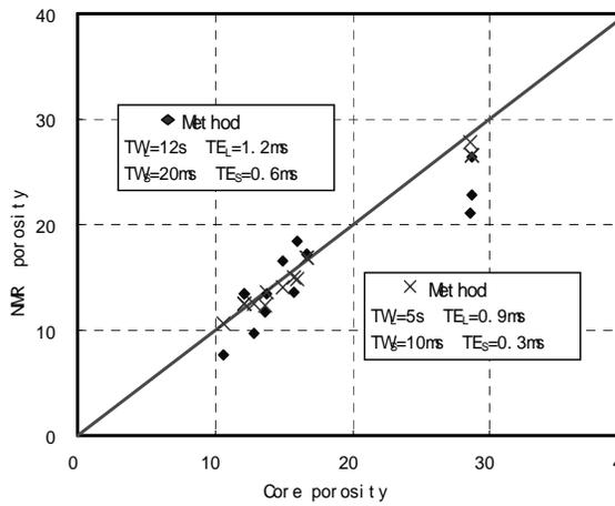
Figure 3. The contrast of NMR porosity and core porosity in sandstones in Xinjiang
