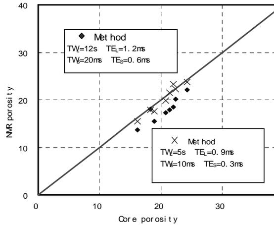
Figure 4. The contrast of NMR porosity and core porosity in sandstones in Dagang
