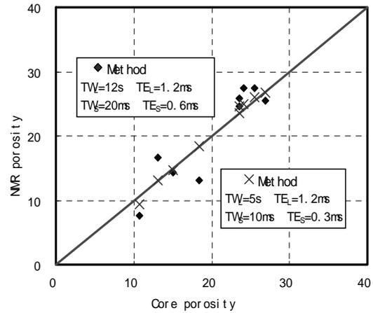
Figure 2. The contrast of NMR porosity and core porosity in sandstones in Daqing
