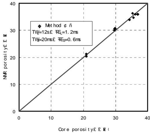
Figure 1. The contrast of NMR porosity and core porosity in artificial ceramic and Berea sandstones
