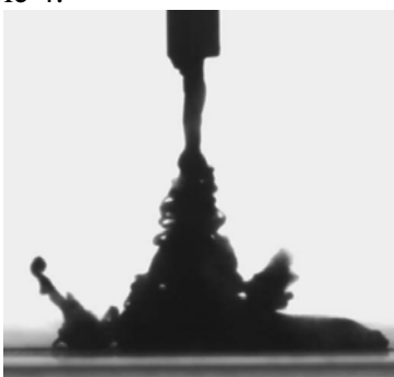
Figure 3. Minnelusa-02 crude oil metered slowly into n-decane forms rigid structures and does not mix. The rectangular feature at the top is a needle with OD of 1.07 mm and ID of 0.70 mm.
