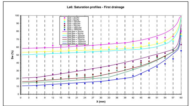
Figure 6. Measured equilibrium saturation profiles – La6 first drainage
