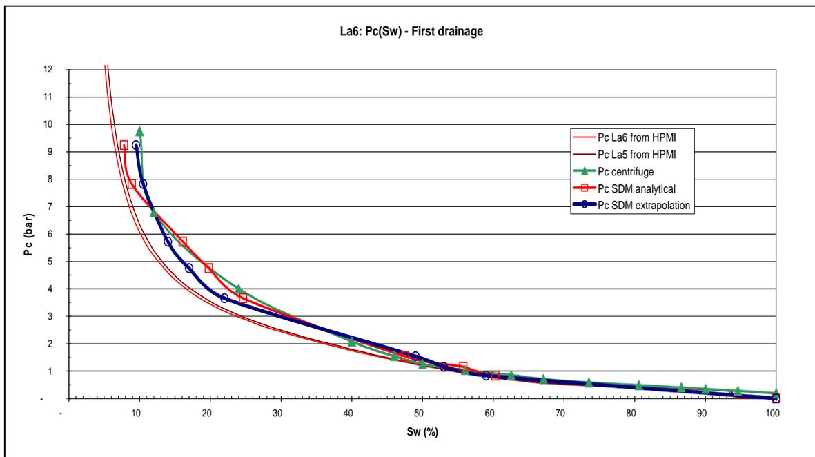
Figure 3. Pc-curves determined by HPMI, centrifuge and SDM methods – La6 first drainage (triangles for centrifuge, squares and circles for SDM, lines for HPMI)
