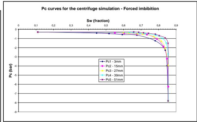
Figure 14. Selection of 5 Pc-curves for the La6 centrifuge numerical imbibition
