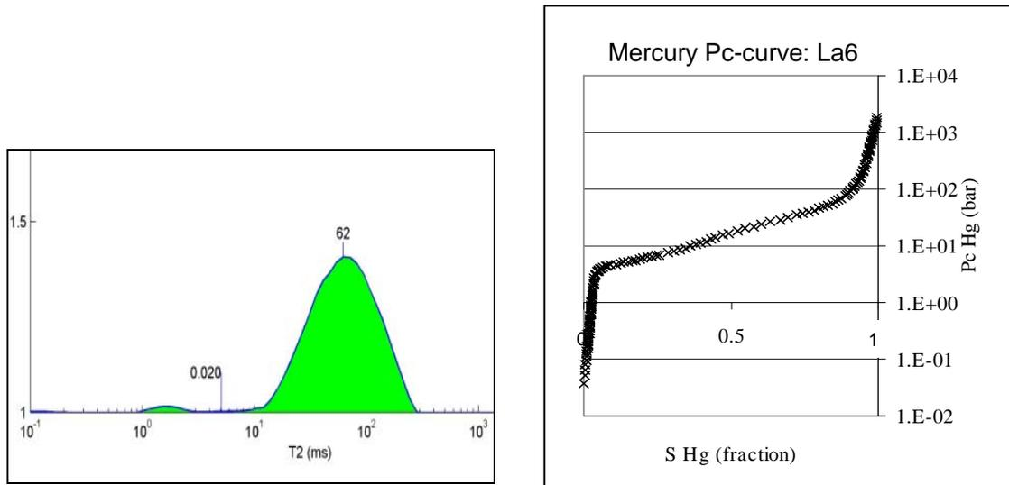
Figure 1. NMR T2 distribution and mercury Pc-curve of La6 plug
