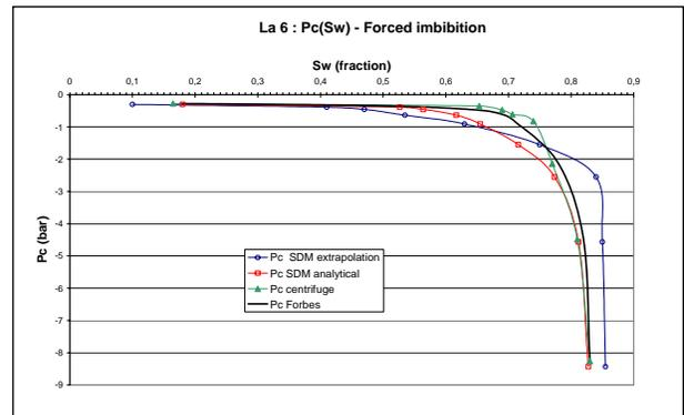
Figure 17. Simulated equivalent homogeneous centrifuge Pc-curve and experimental centrifuge and SDM Pc-curves
