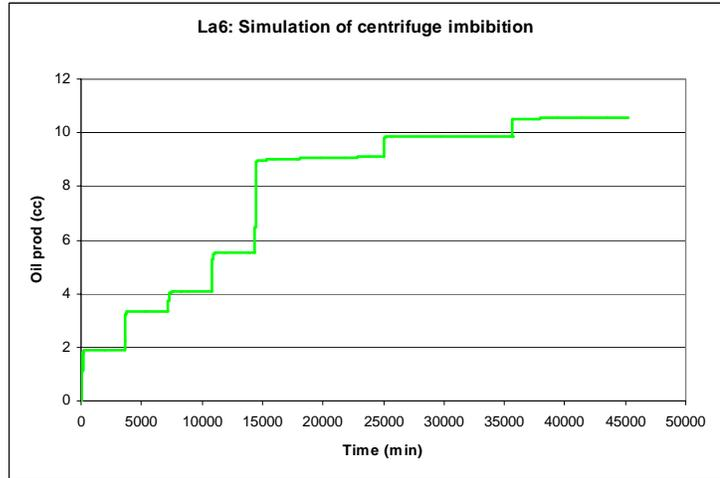
Figure 15. Simulation of La6 centrifuge imbibition - Oil production
