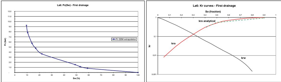
Figure 4. Pc and Kr-curves used for the heterogeneous approach – La6 first drainage
