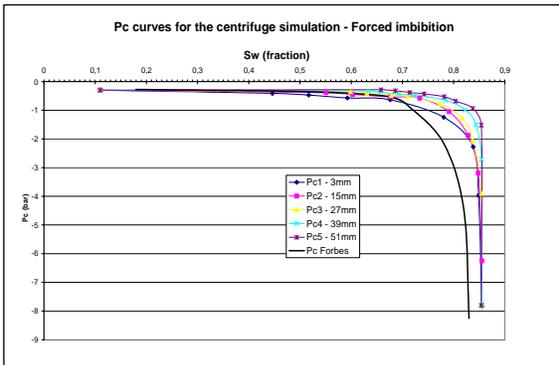
Figure 16. Simulated equivalent homogeneous centrifuge Pc-curve (Forbes) and selected local Pc-curves
