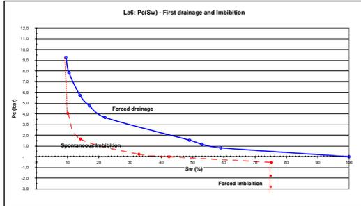
Figure 8. La 6 (WW) - First drainage and imbibition SDM Pc-curves
