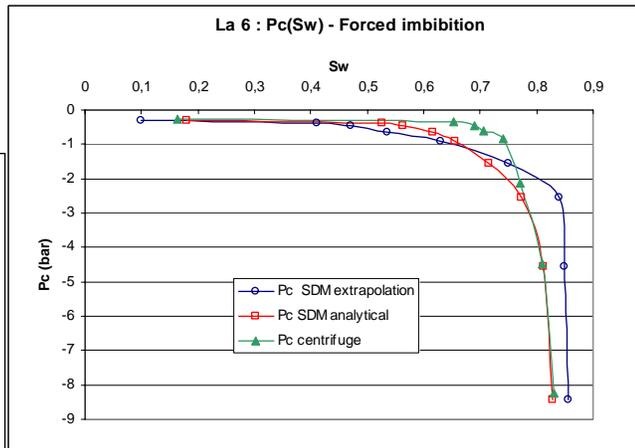
Figure 9. Pc-curves determined by centrifuge and SDM methods – La6 (OW) imbibition
