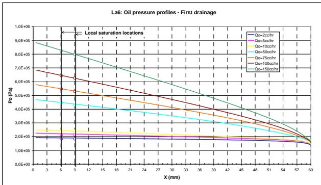
Figure 5. Calculated equilibrium pressure profiles – La6 first drainage
