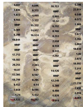
Figure 2: An example mini-permeameter measurement on Natih formation core. The permeability unit is in mD. NMP refers to “no measurement possible”.
