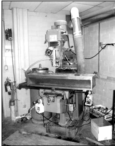
Figure 1. Milling machine used to mill plugs. Note dry-ice trough on table used to keep core frozen with dry-ice.
