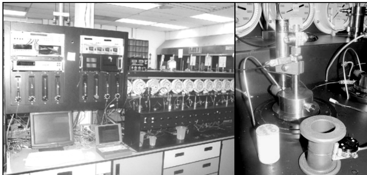
Figure 3. Left, automated porosity permeability isostatic stress cells. Right, flanged viton sleeve with internal radial strain gage and axial LVDT attached to load piston.
