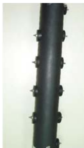
Figure 1. Rubber sleeve with soil column and built-in rod electrodes.
