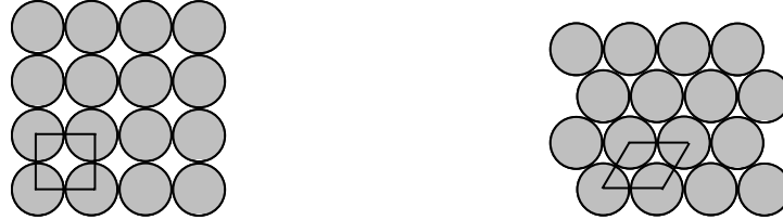
Figure.1 Cubic packing (left plot, porosity 0.48) and rhombohedral packing (right plot, porosity 0.26) of uniform spheres.
