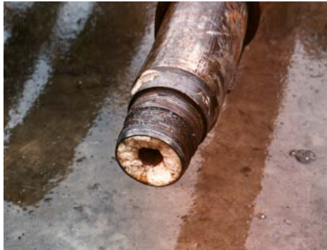
Fig.1: Scale deposition in a pipe
