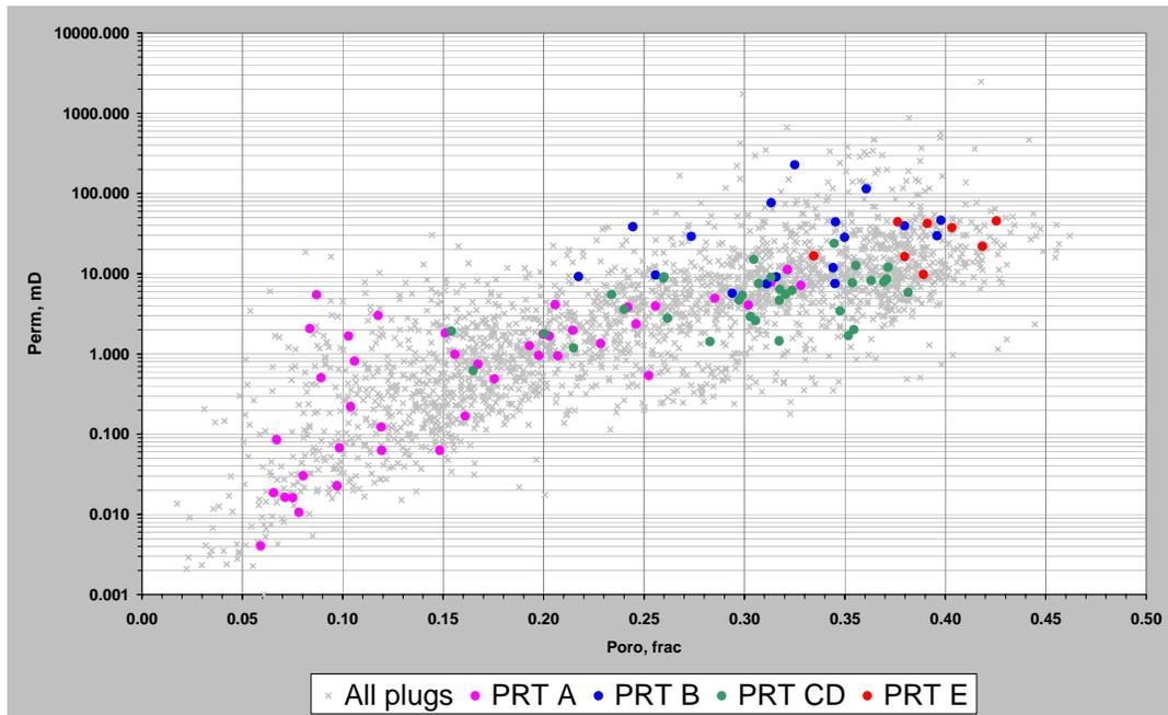
Figure 3. Poro-perm distribution indicating PRT classification. The grey points indicate all available measurements and coloured points indicate samples that have PRT classification.
