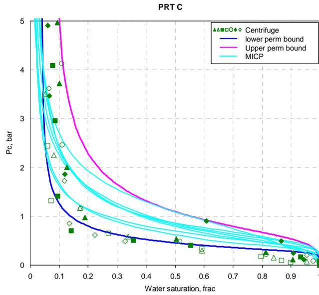
Figure 4. Drainage capillary pressure curves (centrifuge and MICP) fitted with low and high models for PRT C.
