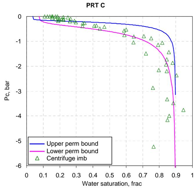
**Figure 6. Imbibition capillary pressure curves. The marked curves are centrifuge measurements and blue and red are the calculated (from drainage using a contact angle of  $125^\circ$ ) high and low curves respectively.**
