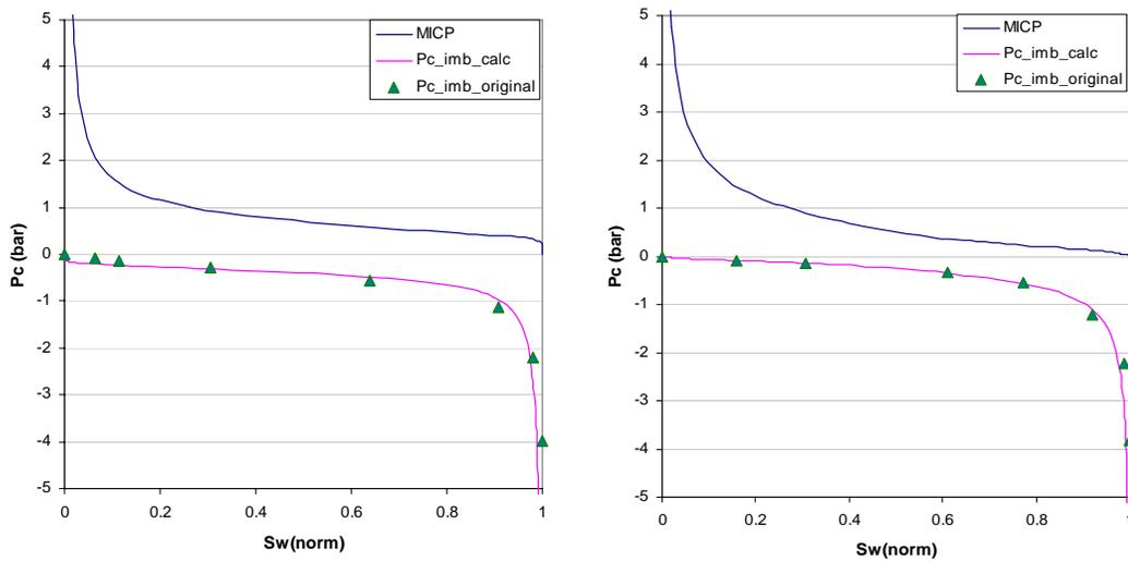
Figure 5. Two examples of plugs used for contact angle calculation. Blue line is the MICP curve, green marks are normalised imbibition capillary pressure curves from centrifuge and red is calculated curve from MICP drainage to get the contact angle.
